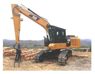
Figure 8: Typical forestry excavator (non-self-levelling) with grapple on a 'high and wide' carrier.
