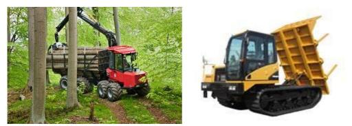
Figure 9: An example of a forwarder shown on the left, and the tracked 'dumper' on the right.
